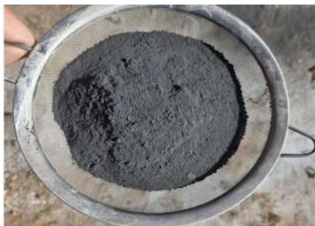
Figure 2 – Galena and sphalerite mineralisation percussion chips intersected in BTPRC010 (81 – 82m), grading 301.6 g/t Ag, 22.47% Pb, 4.61% Zn and 4.6 g/t In.
