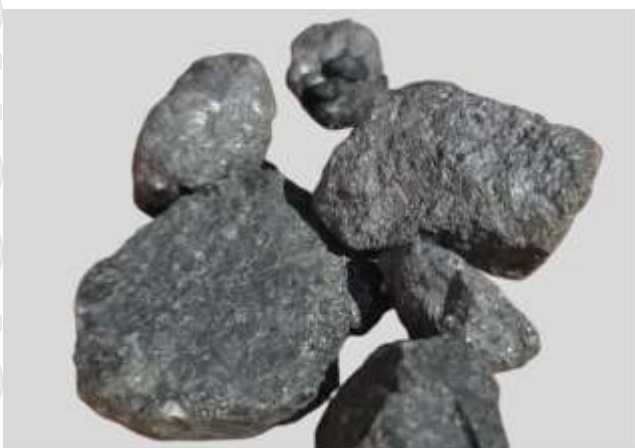
Figure 2 – Galena and sphalerite mineralisation percussion chips intersected in BTPRC010 (81 – 82m), grading 301.6 g/t Ag, 22.47% Pb, 4.61% Zn and 4.6 g/t In.
