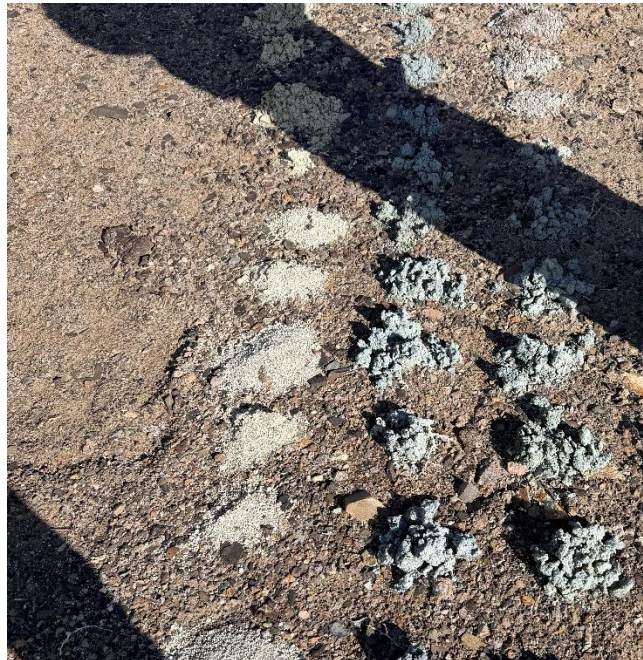
Figure A - 5 Drill cuttings.
