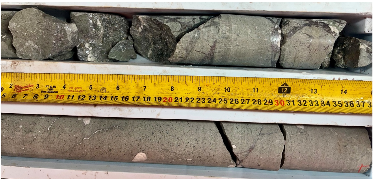
Figure 9 - Chalcocite in crackle breccia cement and surrounding calcite veinlets from 166.4m in DAN26036. Core is NQ2 size.
