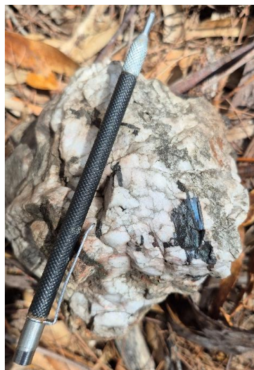
Coarse wolframite crystals hosted by quartz veins at the Lutwyche Prospect, Scamander Project (Samples LW26013 (Left) and LW26006 (Right))
