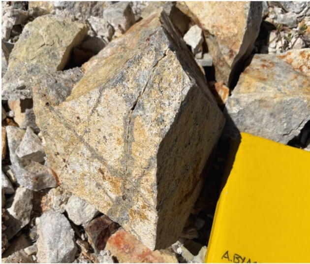
Figure 4: Breccia quartz veins in altered granite.
