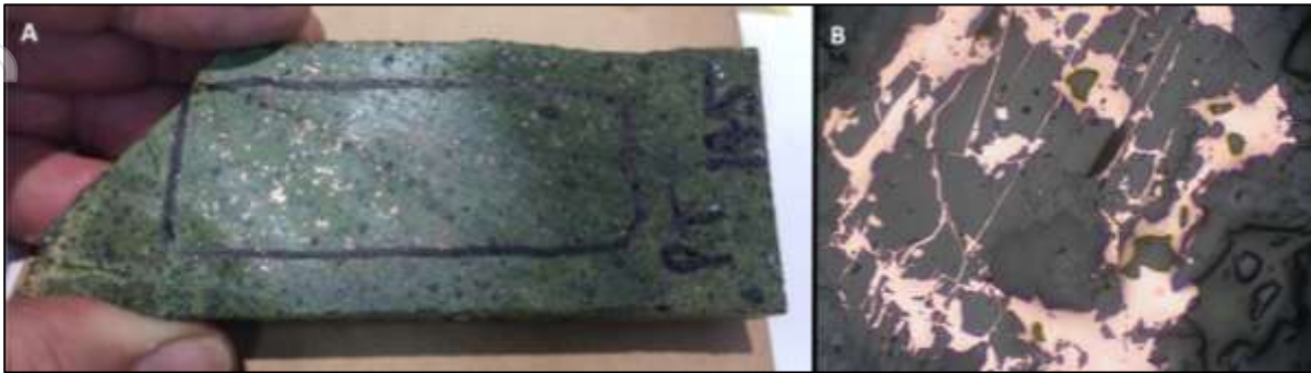
Figure 7: Lyon's Prospect. A) cut field specimen showing pale olive green epidote altered porphyritic basalt with disseminated native copper mineralisation (metallic pale pink). B) Corresponding petrographic section (field of view 2mm) showing pale pink native copper as fracture-controlled replacement of host mineral (pyroxene). This correlates with grab sample GRR00145 reporting 1.94% copper.
