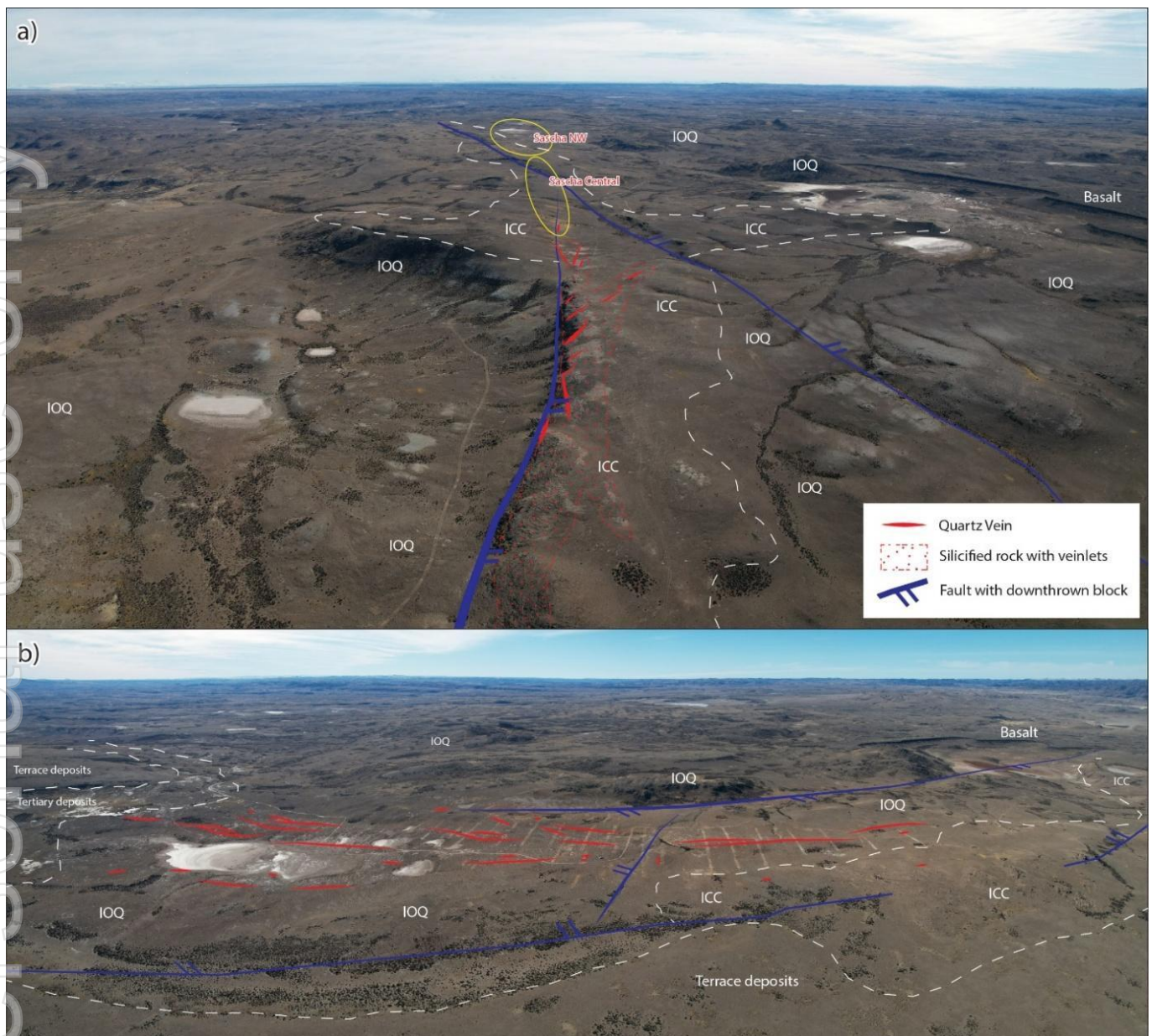
Figure 4 – Aerial views of the main segments of the Sascha Vein System. a) Aerial panoramic view of the Sascha Southeast segment showing the main lithological and structural features of the area. b) Aerial panoramic view of the Sascha Northwest segment showing the main lithological and structural features of the area, including the partial cover by Tertiary deposits and terrace deposits.
