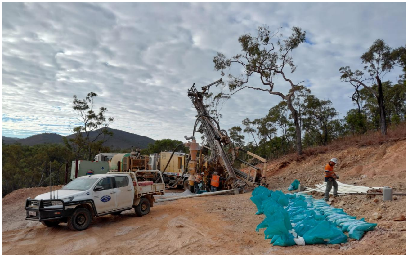
Figure 1 Wheel-mounted RC rig drilling at Union Jack
