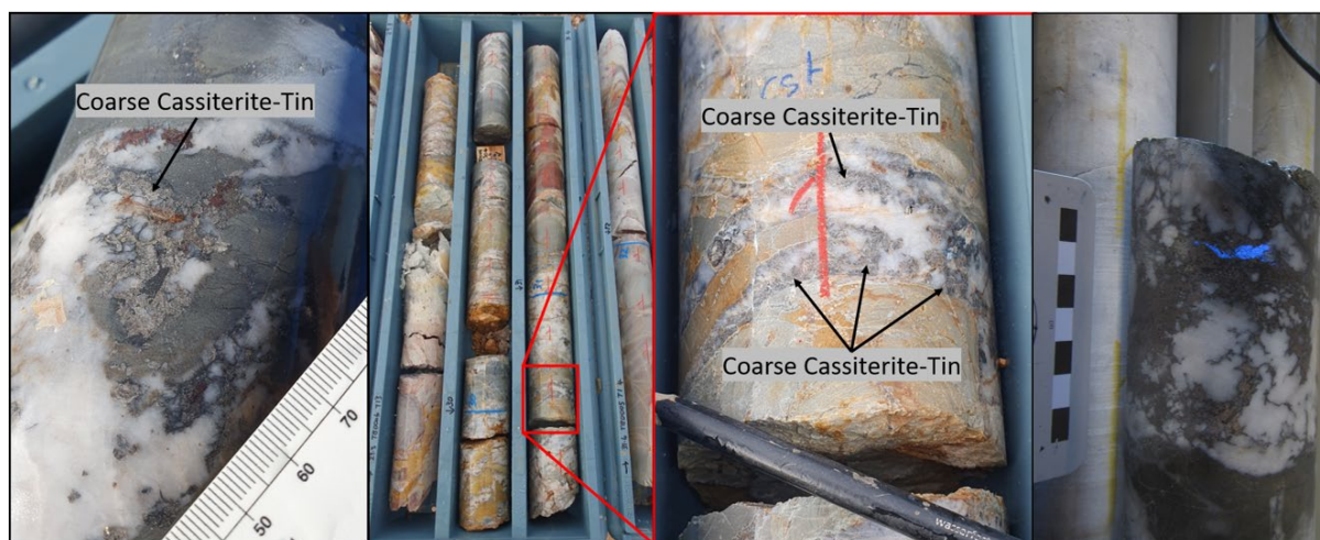
Figure 3 Examples of Coarse tin-tungsten mineralisation at Tallebung
