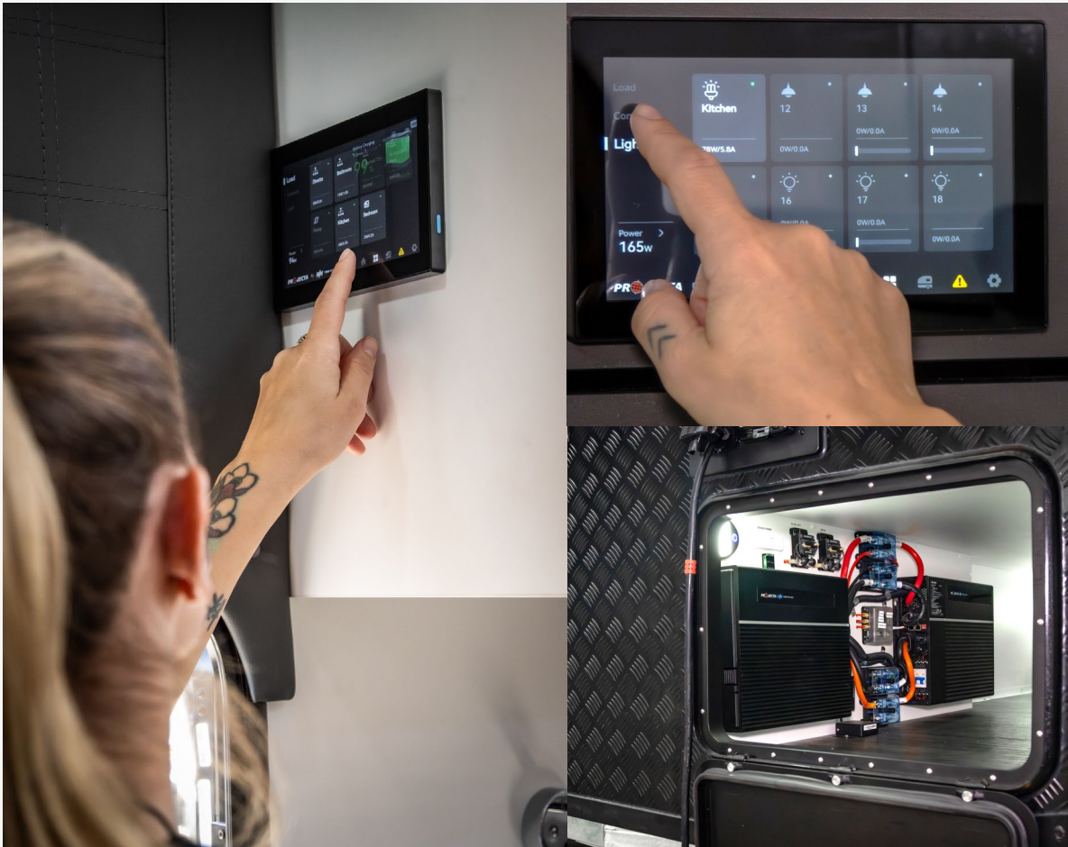
For serious off-grid travel, Projecta's Intelli-Grid 48V power management system delivers up to 4,000W of continuous power to smoothly run high-demand appliances. Moving from 12V to 48V enables the same power to be delivered while using lower current resulting in greater efficiency and less strain on components
