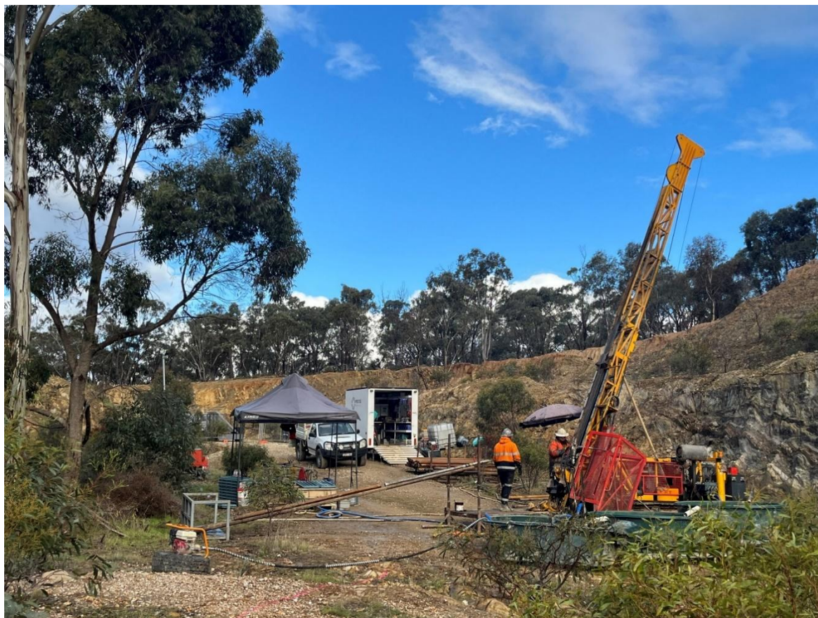
Figure 4 - Diamond Drilling within the Walkers pit at the Comstock Gold Project. Picture taken June 2026 and shows rig targeting shallow depth drilling on the Walkers stockwork vein area and utilizing the existing pit access ramp.
