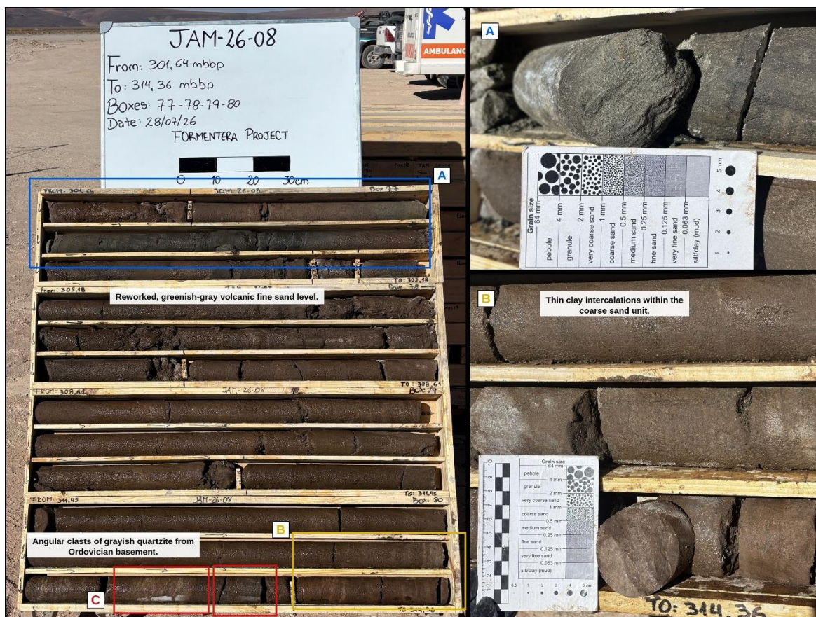
Figure 2. Core from 301-314m showing visual high porosity core sand unit.
