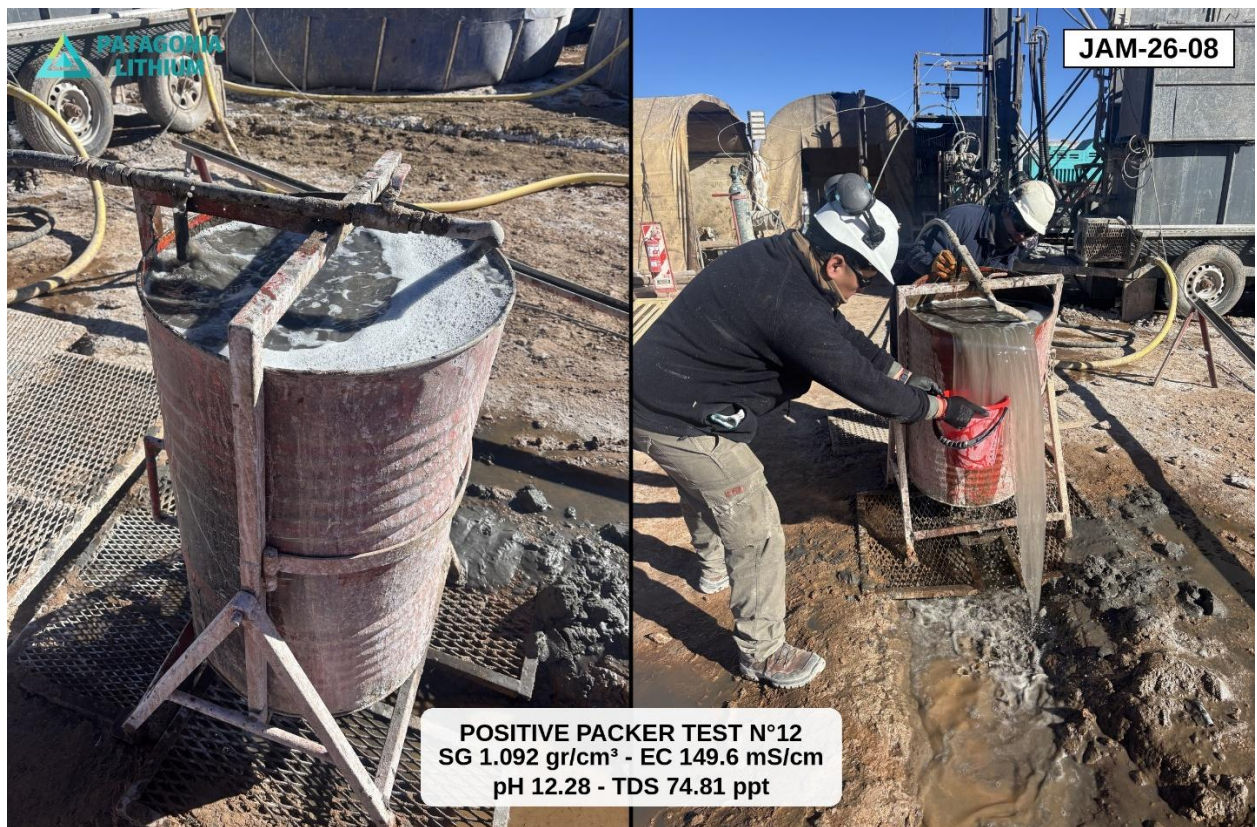
Figure 7. Packer test 12 – 10 th successful test showing high flow rate from pump.
