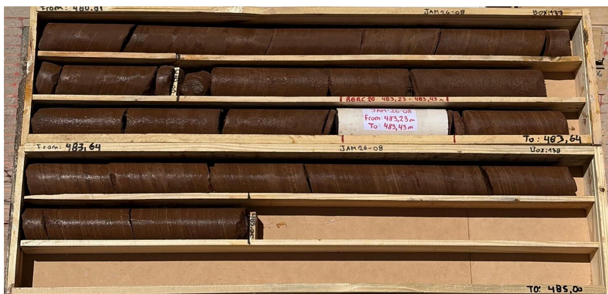
Figure 3. Drill core from last 5 metres (480-485m) showing consolidated clays.
