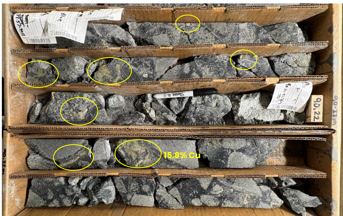
Figure 1: Visible chalcopyrite copper mineralisation in tourmaline breccia between 89–91m at the end of hole DD26CT008 with a spot pXRF copper assay.
