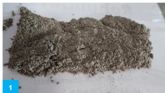
Figure 5: 1. Pulverised spent catalytic converter; 2. Conventional flowsheet for catalytic converter processing (Yakoumis, I., et al. 2021)
