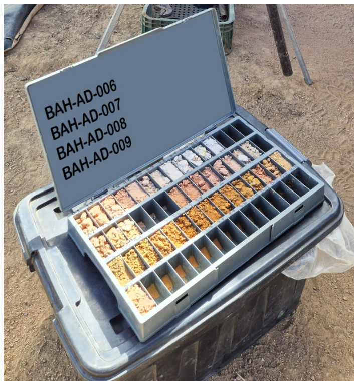
Figure 4A and 4B: Samples are collected from barrel (BAH-AD-0009) and preserved in chip trays
