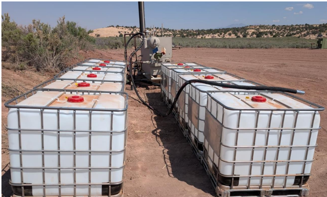
Figure 2: Lithium brine storage totes
