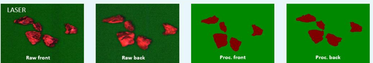
Figure 2. Ore sorting of various metallurgical sample types from Big Jim by TOMRA. Both Laser and XRT Technology clearly differentiates between ore and waste types
