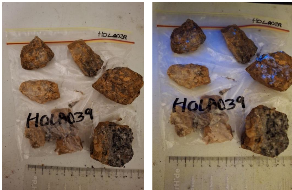
Figure 1: Sample HOLA039 grading 12.45% W (15.69% WO_3 ) – under normal (left) and UV(right) light
