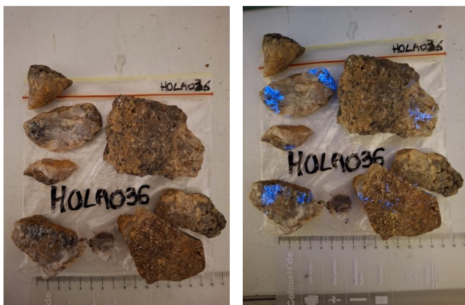
Figure 2: Sample HOLA0036 grading 6.16% W (7.76% WO_3 ) – under normal (left) and UV(right) light
