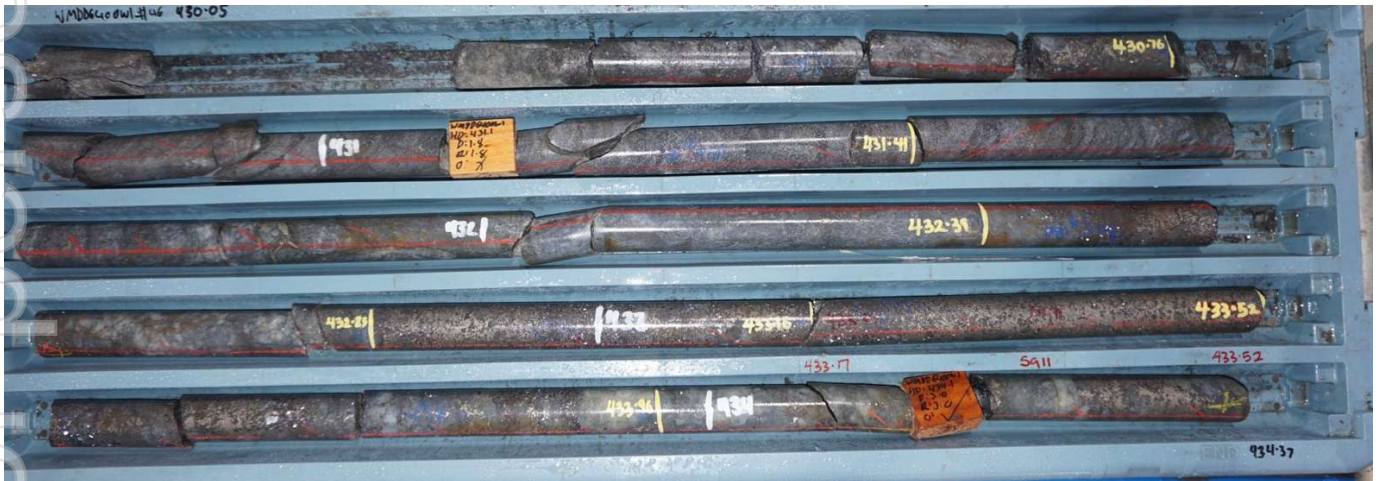
Figure 2 – WMDD6400W1 core, inc. sections from intercept assaying 5.4m at 19.5% ZnEq, 540g/t AgEq from 432.4m
