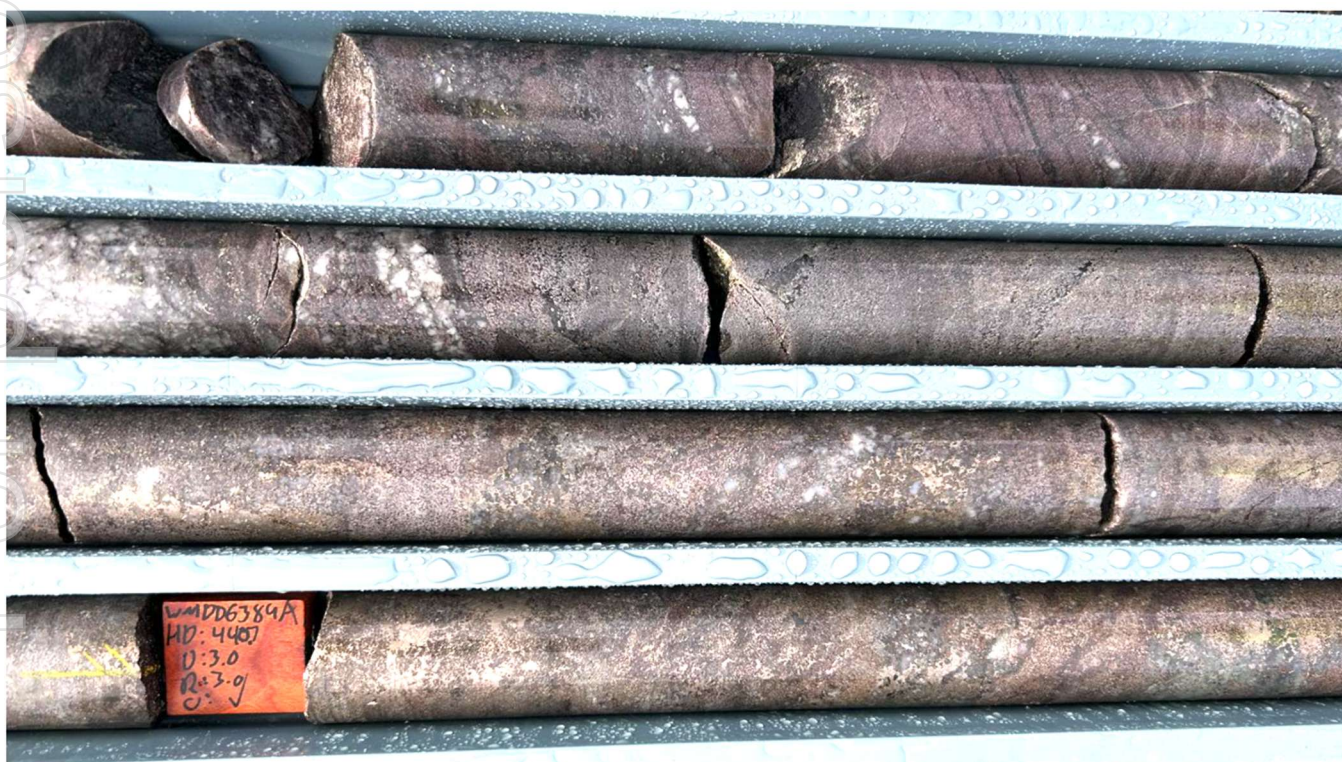
Figures 4, 5 & 6 – WMDD6389A drill core, showing an extensive intercept of a zone of mineralisation up to 35m thick (assays pending)
