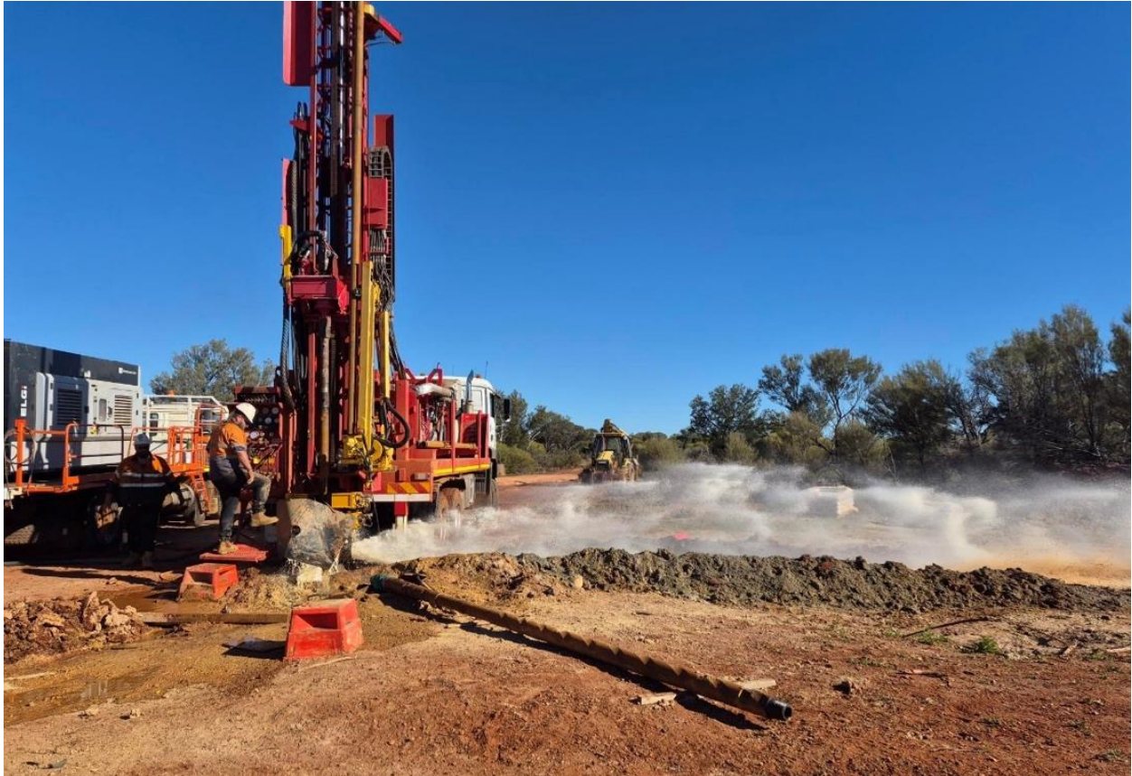
Figure 1: Water bore drilling Mulgabbie North
