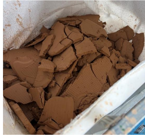
Figure 15: Filter cakes produced during vendor testwork (left) and by the demonstration plant filter (right).
