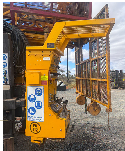
Fall protection fitted over driller's control panel on a diamond rig.
