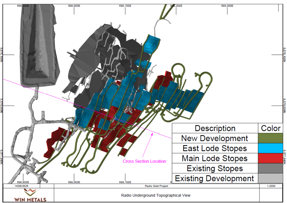
Figure 12: Proposed underground development and stopes
