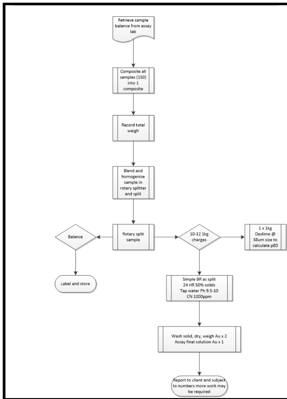
Figure A3: Princess Royal metallurgical testwork flowsheet
