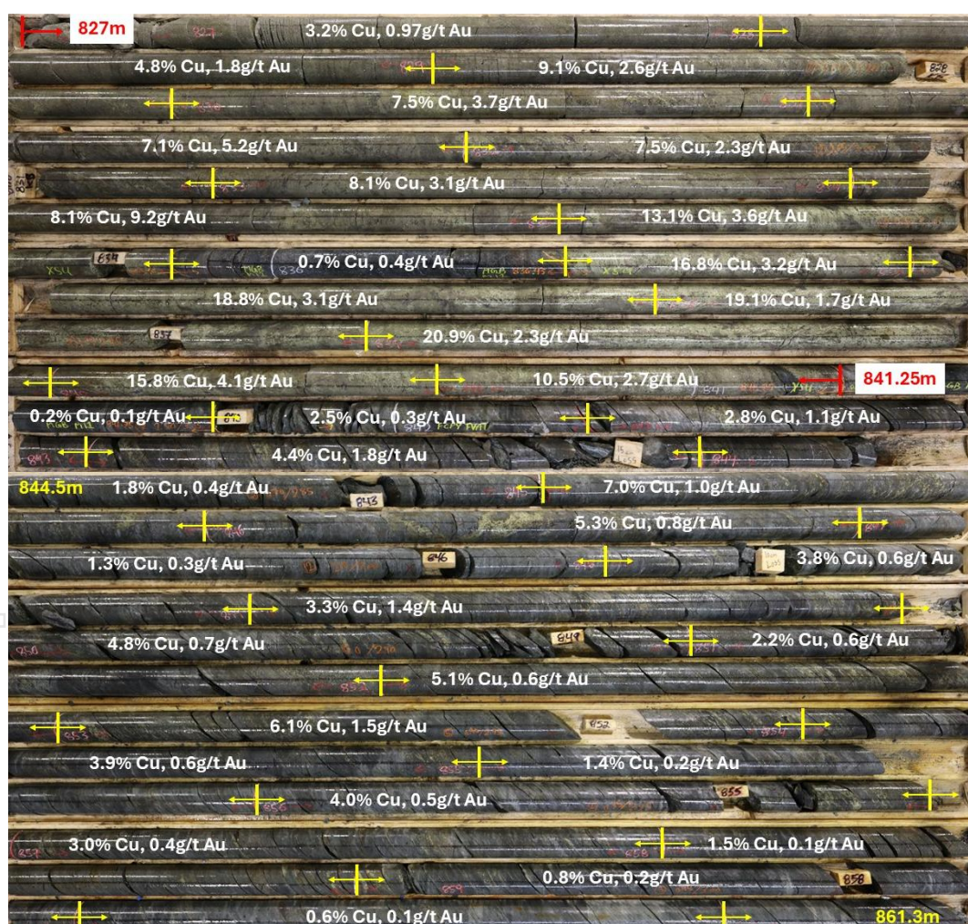
Figure 31: Core photographs for MUG25-202 showing the high-grade Core Zone. This convergent zone consists of the upper VMS zone (827m-841.25m) that grades 14.3m @ 13.7% CuEq and the adjacent broad FWZ stringer-style mineralisation. This is part of the broader step-out intersection of 49.0m @ 6.1% CuEq that is the deepest hole drilled into the Ming Deposit to date.
