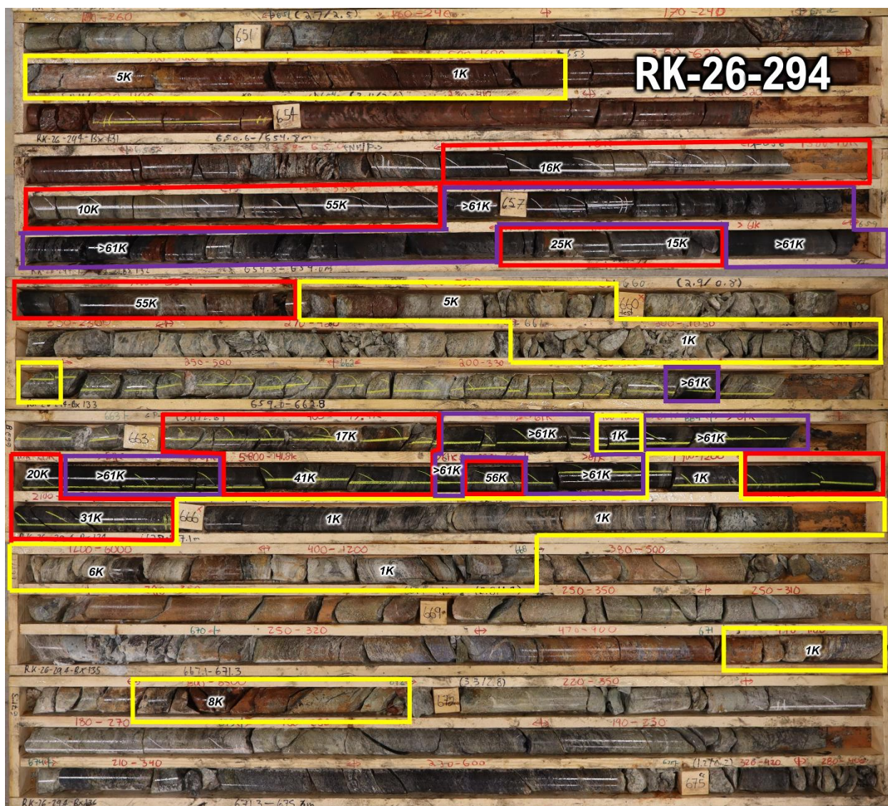
Figure 3: Core photo from RK-26-294 displays cumulative 3.1 m of off-scale (>61,000 cps) uranium mineralization between 656.9 and 665.4 m down hole; yellow outlines >1,000 cps, red outlines >10,000 cps, >61,000 cps outlined in purple
