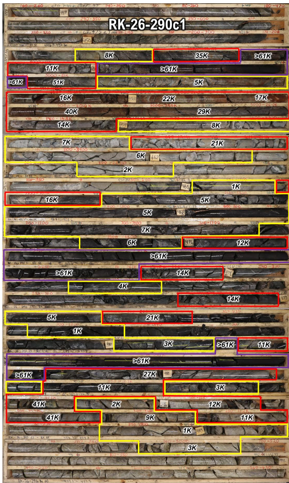
Figure 4: Core photo from RK-26-290c1 displays cumulative 5.2 m of off-scale (>61,000 cps) uranium mineralization between 451.4 and 491.4 m down hole; yellow outlines >1,000 cps, red outlines >10,000 cps, >61,000 cps outlined in purple
