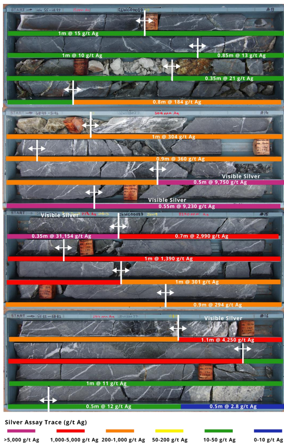
Figure 3. Diamond drill cut core photograph of 26WCDD037 from 44.55m to 58.82m downhole depth highlighting visible native silver hosted in fracture fill quartz-carbonate veining within ultramafic, and corresponding assay results (See Appendix 3). Note the assay value quoted as 0.5m @ 2.8 g/t in the final interval depicted is from an interval that continues into the next core tray in the sequence but not included in this image.
