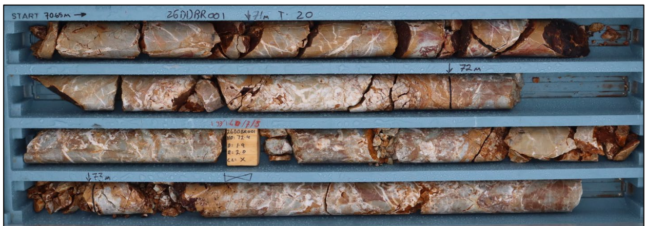
Figure 3: Gold bearing quartz-cemented breccia within interval 14m at 0.4g/t Au and 5g/t Ag from 61m in 26DDBR001 (weathered/oxide zone).
