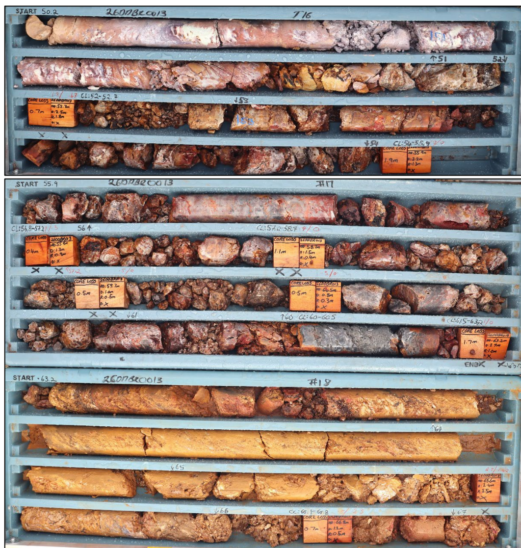
Figure 4: 26DDBR013 high-grade gold-bearing drill core, 13.6m at 4.6g/t Au & 23g/t Ag from 51.4m (50% recovery).
