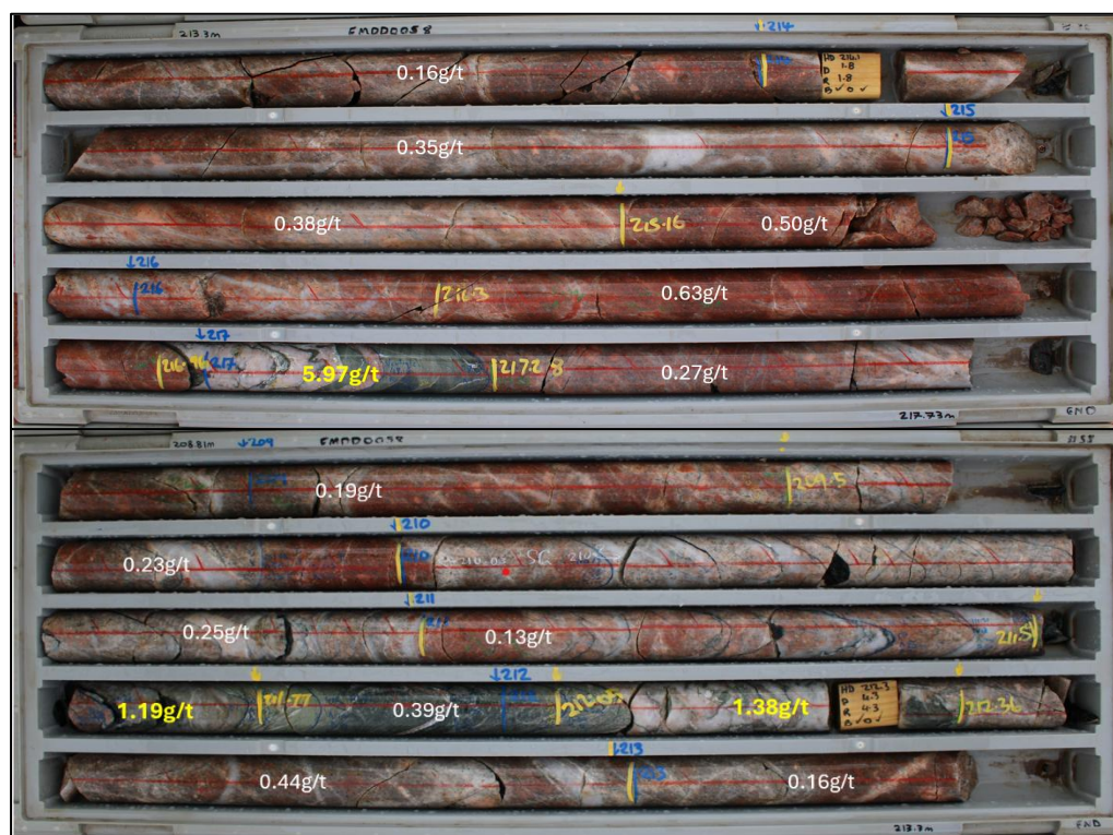
Figure 5: Core tray photos from FMDD0058 208.81-217.73m with gold grade overlain and high-grade intercepts in yellow. Demonstrates moderate to strong silica-carbonate alteration of the sheared quartz syenite intruded with N-S trending lamprophyre lenses bookended with massive quartz veining associated with high grade gold.
