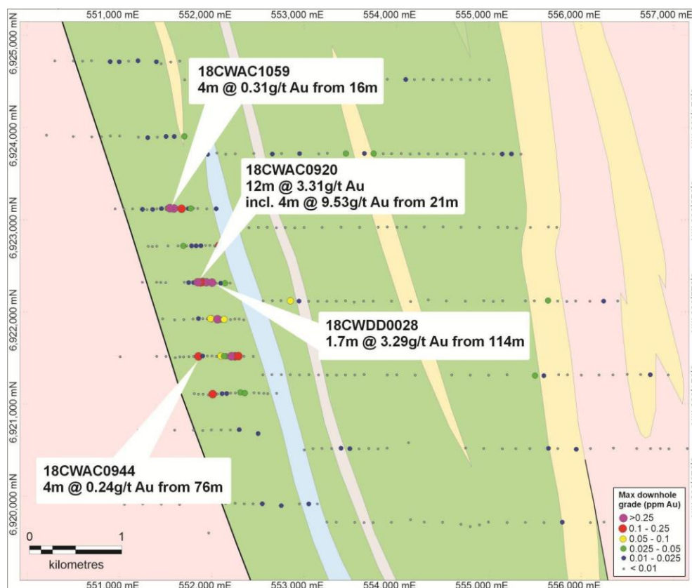
Figure 2: Bloodwood prospect – historical drill hole locations coloured by maximum downhole gold grade, with significant intercepts annotated. Gold anomalism is coherent over approximately 5km of strike.
