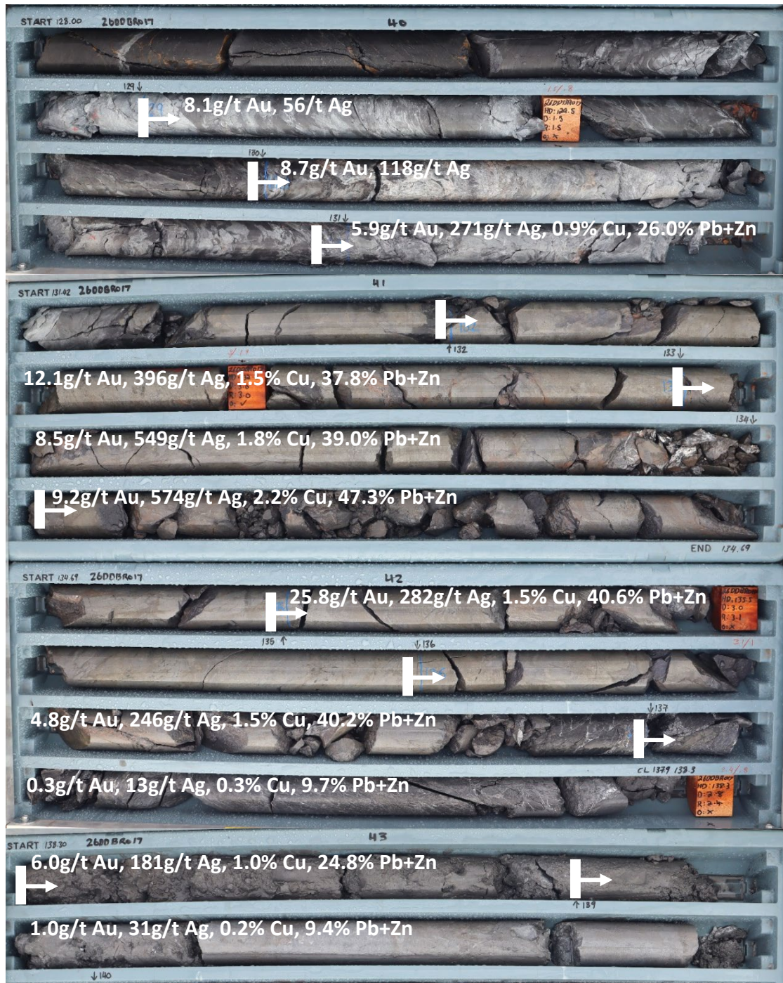
Figure 1: Discovery hole 26DDBR017, showing consistently high-grade down hole gold-silver-base metals assays from 129m to 139m, which includes 8m at 10.4g/t Au, 311g/t Ag, 1.2% Cu & 29.0% Pb+Zn fm 129m.
