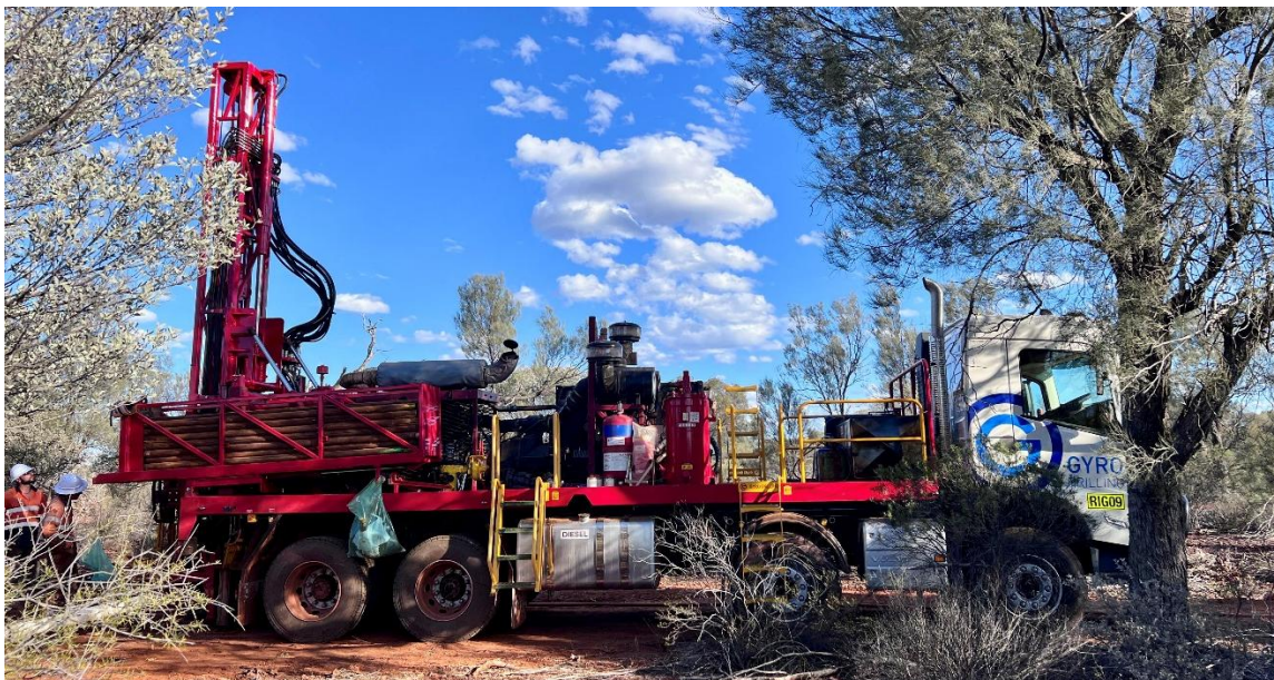
Figure 1: Photo of air core drilling at Illara.
