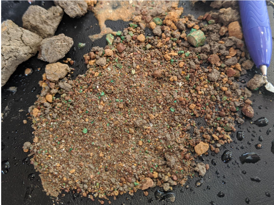
Photo 2 – Copper Carbonate (Malachite) mineralisation in historical water bore at Jessica: 0-3m from RN28419 – chemical assay 1.5% Cu
