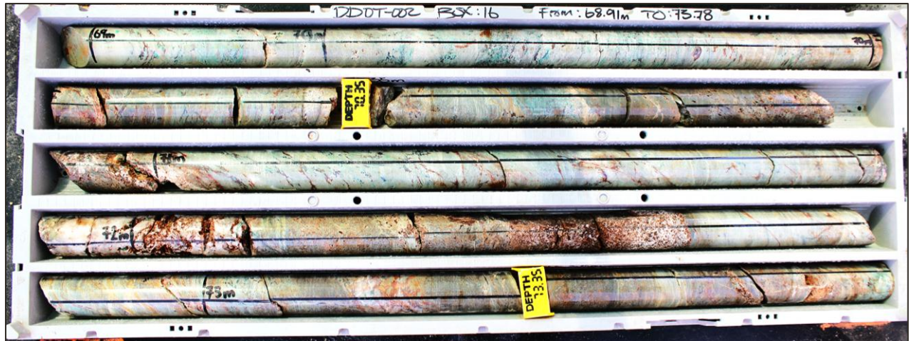
Figure 2 – DDOT002 Core Box 15 from 64.1 to 68.91m and Core Box 16 from 68.91 to 73.78m (refer to Appendix A for details of visual estimates of mineralisation). Refer to cautionary note on page 2 above regarding visual estimates of mineralisation.
