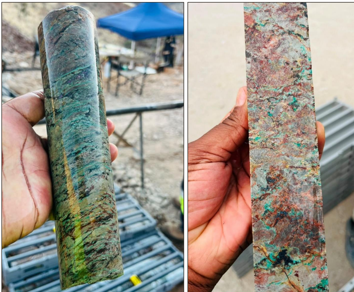
Figure 1 - DDOT002 Core from 68.13m to 68.34m showing disseminated malachite, chrysocolla, cuprite and chalcocite mineralisation (left) and DDOT001 Core from 64.03m to 64.17m showing disseminated chalcocite, cuprite and diopside mineralisation (right). Refer to Appendix A for details of visual estimates of mineralisation.
