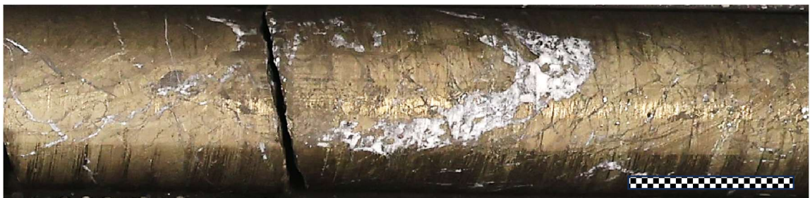
Figure 1. Semi massive iron and copper sulphides at 147.9m depth on drill hole CD26-009. Scale bar = 5cm.
