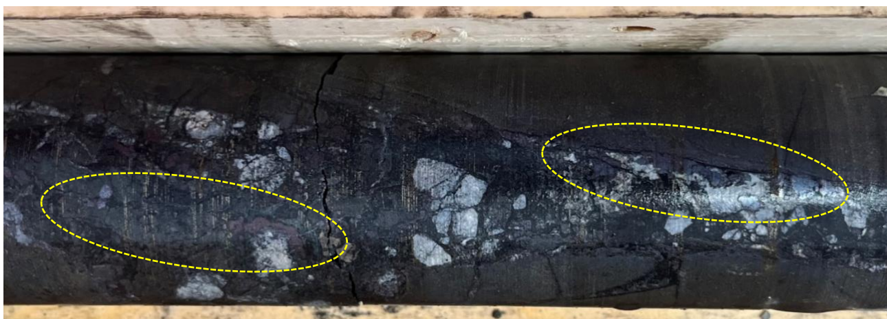
Figure 9 - Photograph of vein and breccia cement hosted chalcocite mineralisation that characterises the sulphides at 81m in DAN26047. Yellow dashed circles outline the bornite and chalcocite mineralisation. Drill core is NQ2 diameter.
