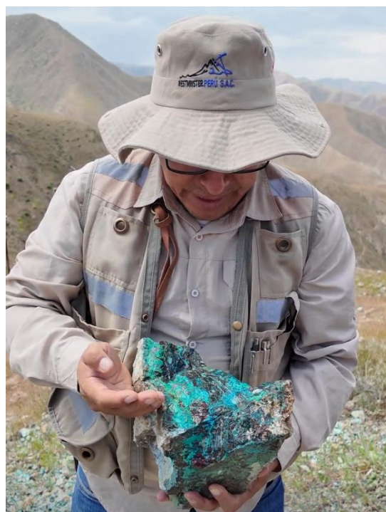
Figure 3: Cinto rock geochemistry. LHS (located proximate to Channel 7, sample 18369, taken across mineralisation in brecciated andesitic tuff exposed by gully erosion. Sample length 1.1m. Assay results: Au 0.535 g/t, Ag 25 g/t, Cu 8.7%, Mo 1 ppm, Pb 283 ppm, Zn 873 ppm 4 , RHS (located proximate to drill
