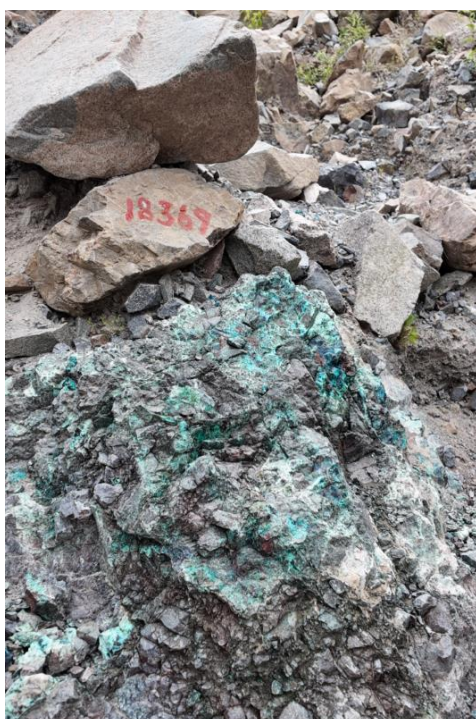
Figure 3: Cinto rock geochemistry. LHS (located proximate to Channel 7, sample 18369, taken across mineralisation in brecciated andesitic tuff exposed by gully erosion. Sample length 1.1m. Assay results: Au 0.535 g/t, Ag 25 g/t, Cu 8.7%, Mo 1 ppm, Pb 283 ppm, Zn 873 ppm 4 , RHS (located proximate to drill
