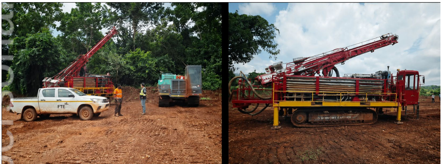
Figure 1. RC drill rig setting up and starting the first hole at the Bondoukou Project.
