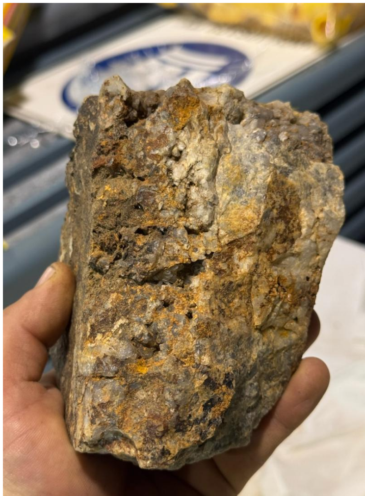
Figure 3: Quartz veining within an area of hydrothermal alteration at eastern Blue, associated with coincident bismuth anomalism and rock-chip gold grades of up to 5.16 g/t Au (RTRK_00322).
