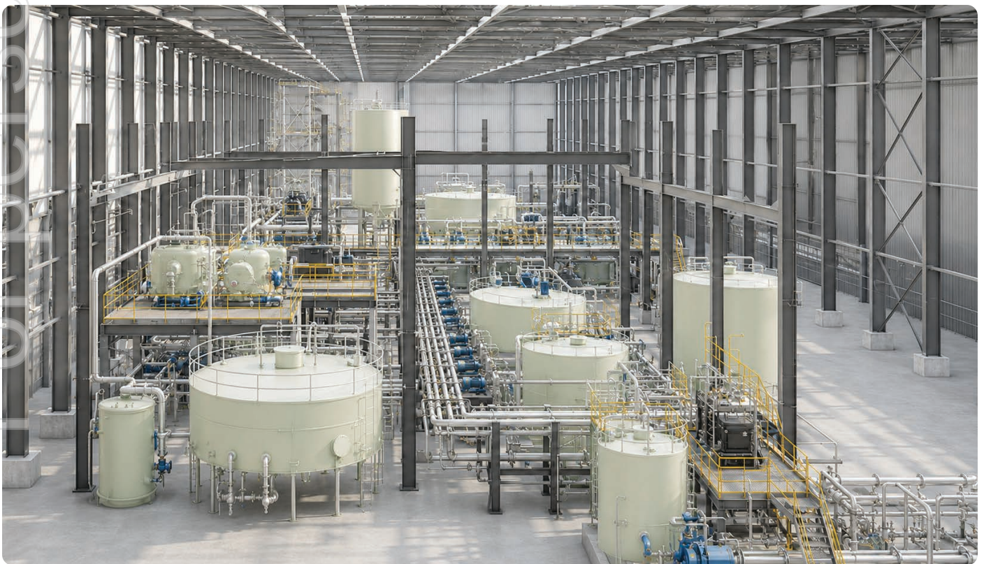
Photo: Lithium Carbonate Precipitation Section – Proposed Brownsville Lithium Refinery (Illustrative)
