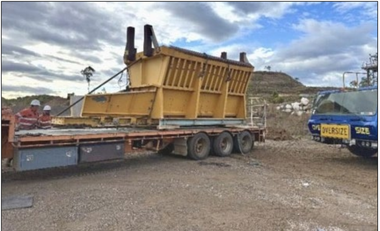
Figure 7: Relocation of mill feed hoppers.
