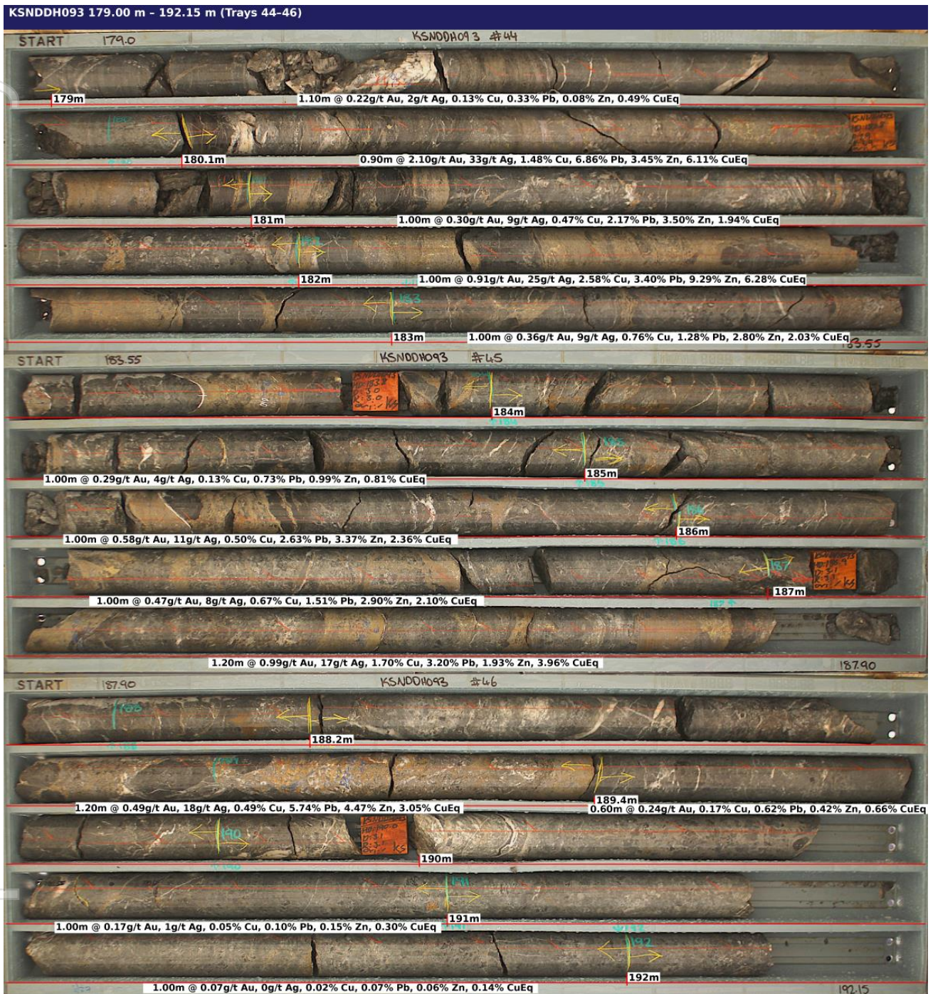
Figure 5: Core photos KSNDH093, 179m - 192.15m, showing chalcopyrite, galena, sphalerite mineralisation.
