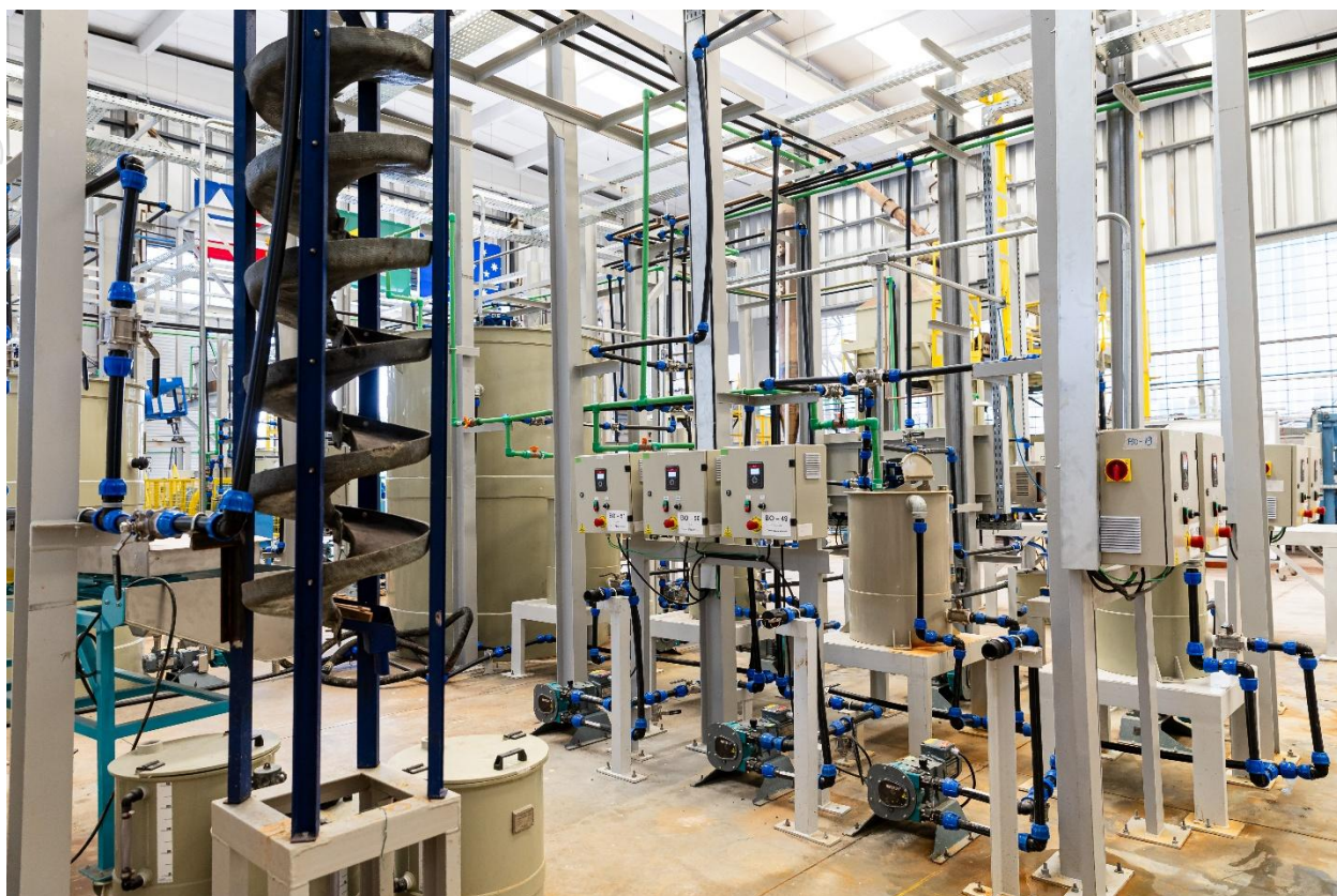
Figure 12: Gravity separation / spiral concentrator.
