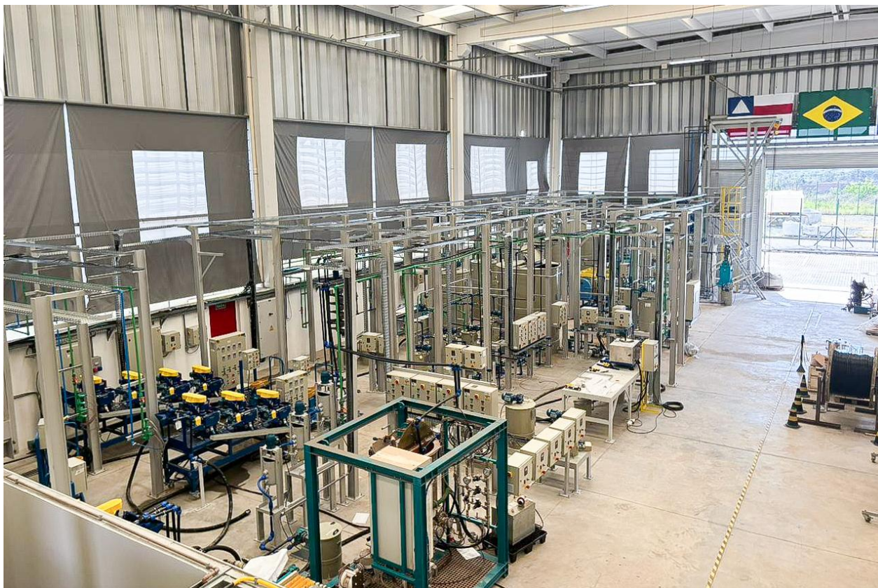
Figure 4: Stage 1 Beneficiation Facility Overview - 100 kg/h Capacity.
