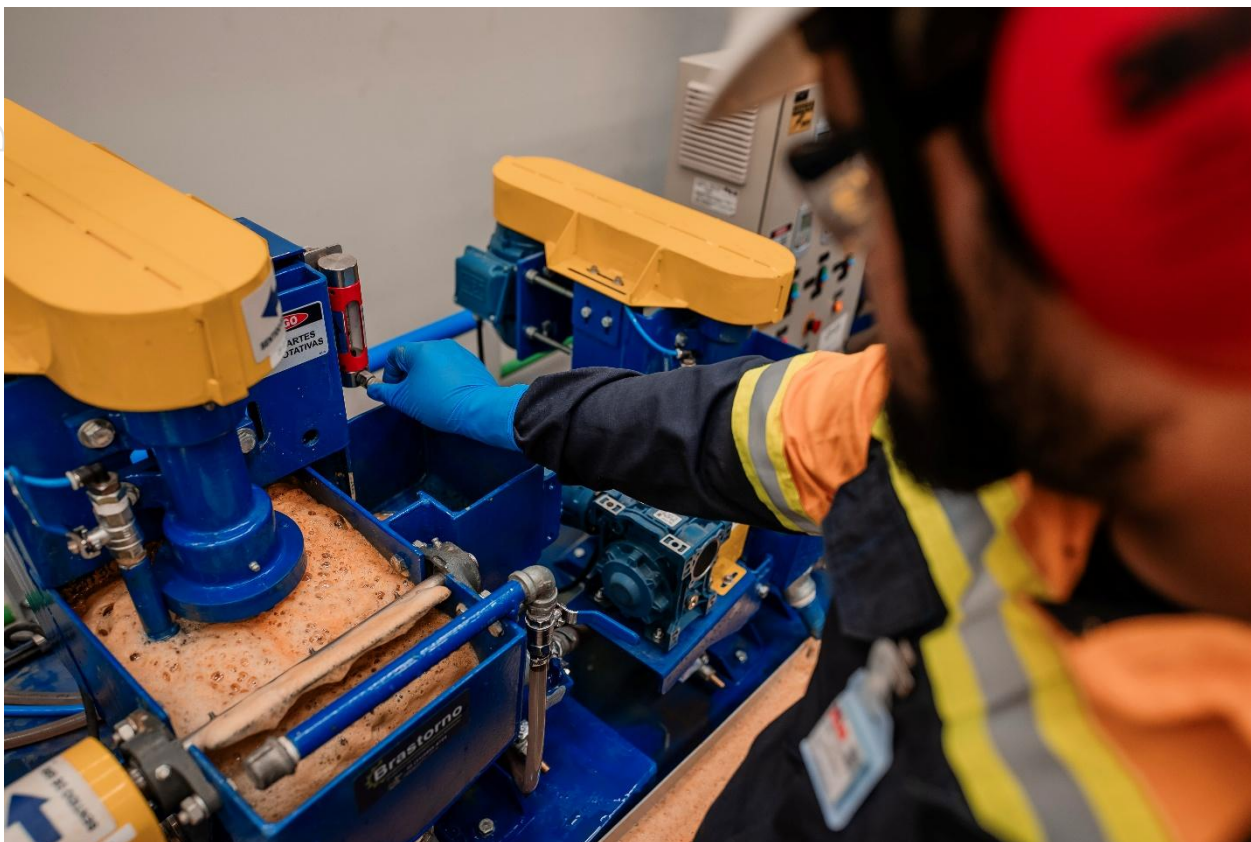
Figure 10: Flotation cell air flow adjustment during commissioning.
