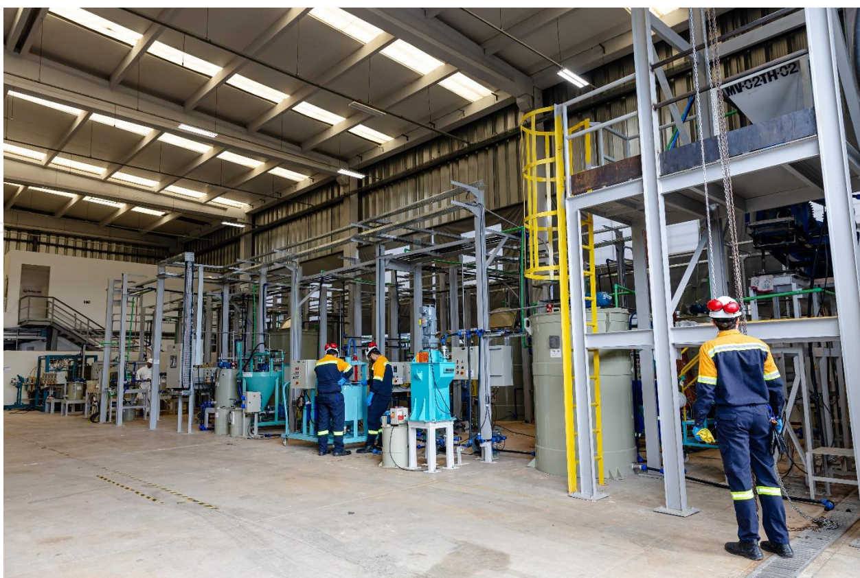
Figure 3: Stage 1 Beneficiation Facility Overview - 100 kg/h Capacity.
