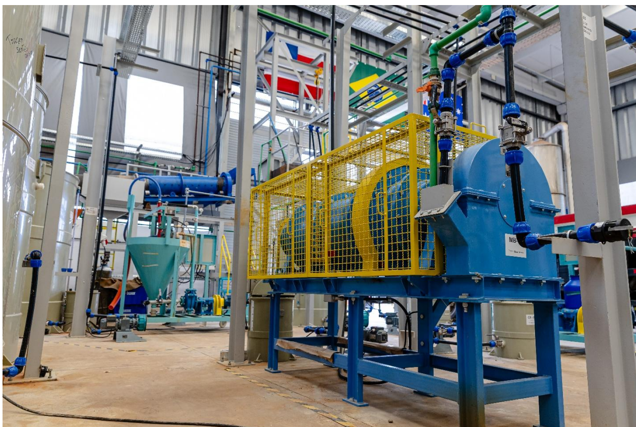
Figure 5: Grinding mill within the Stage 1 beneficiation pilot plant.
