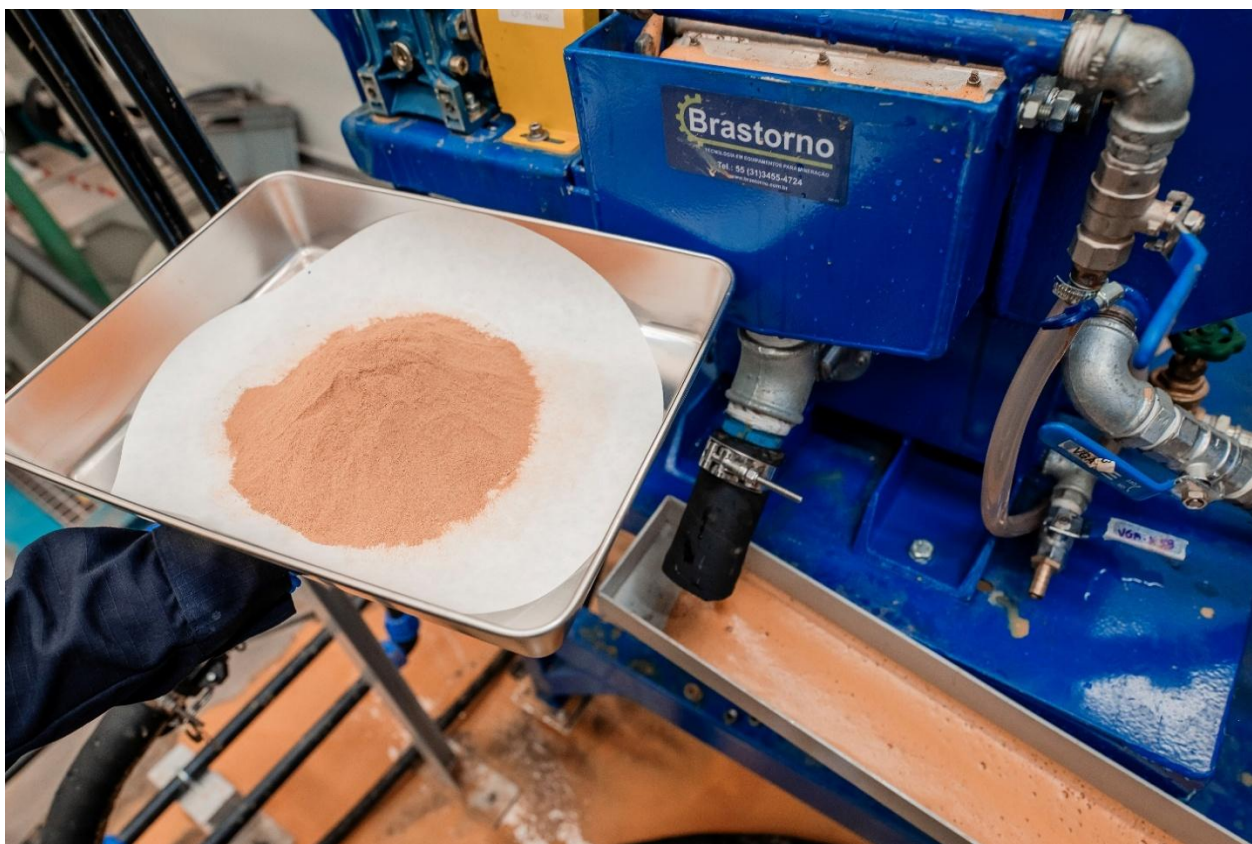
Figure 8: Prepared feedstock for the Stage 1 pilot plant's wet beneficiation circuit.
