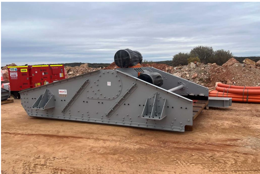
Figure 6: First mechanical equipment delivered to site (vibrating screen)
