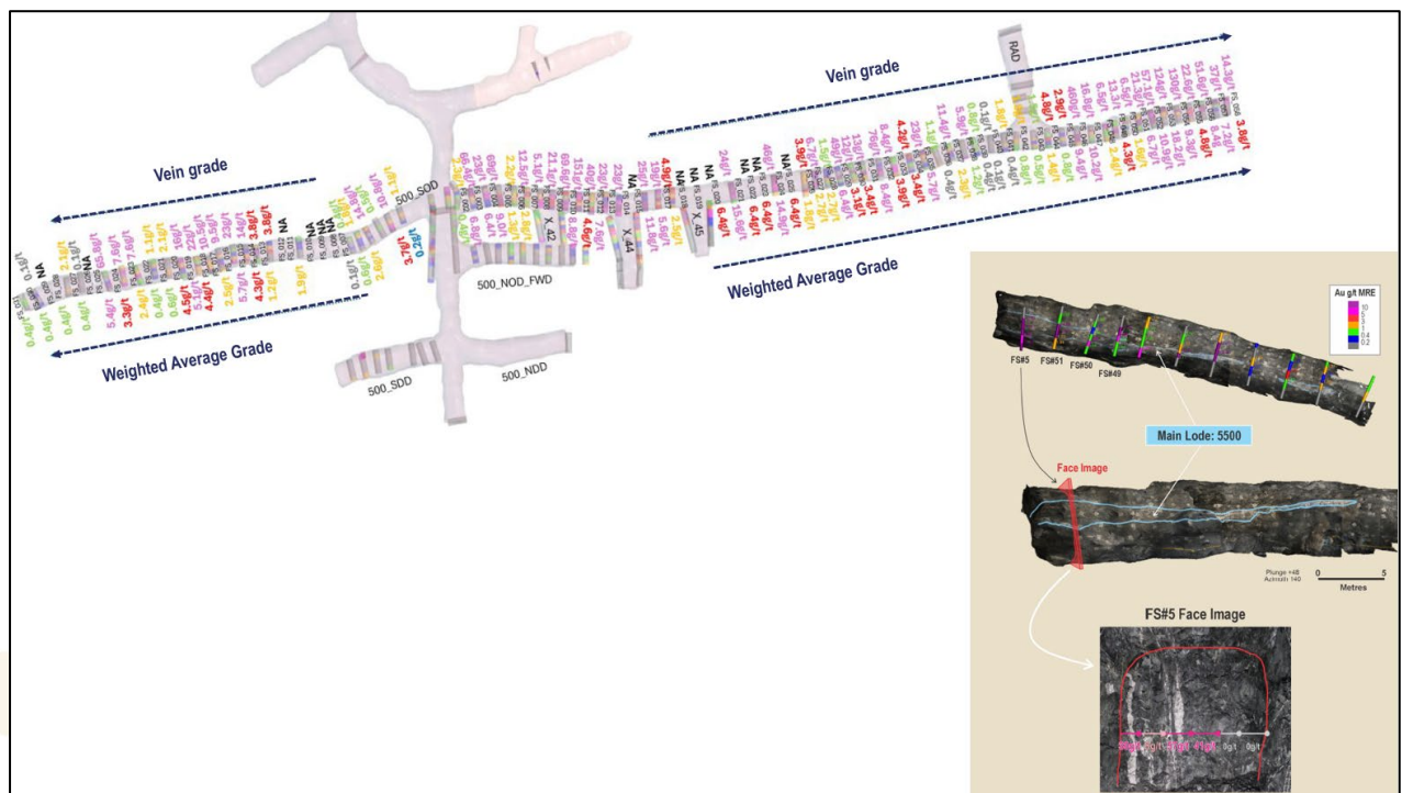
Figure 3 – Face mapping and sampling of Main Lode 500 level – the first level beneath previously mined open pit
