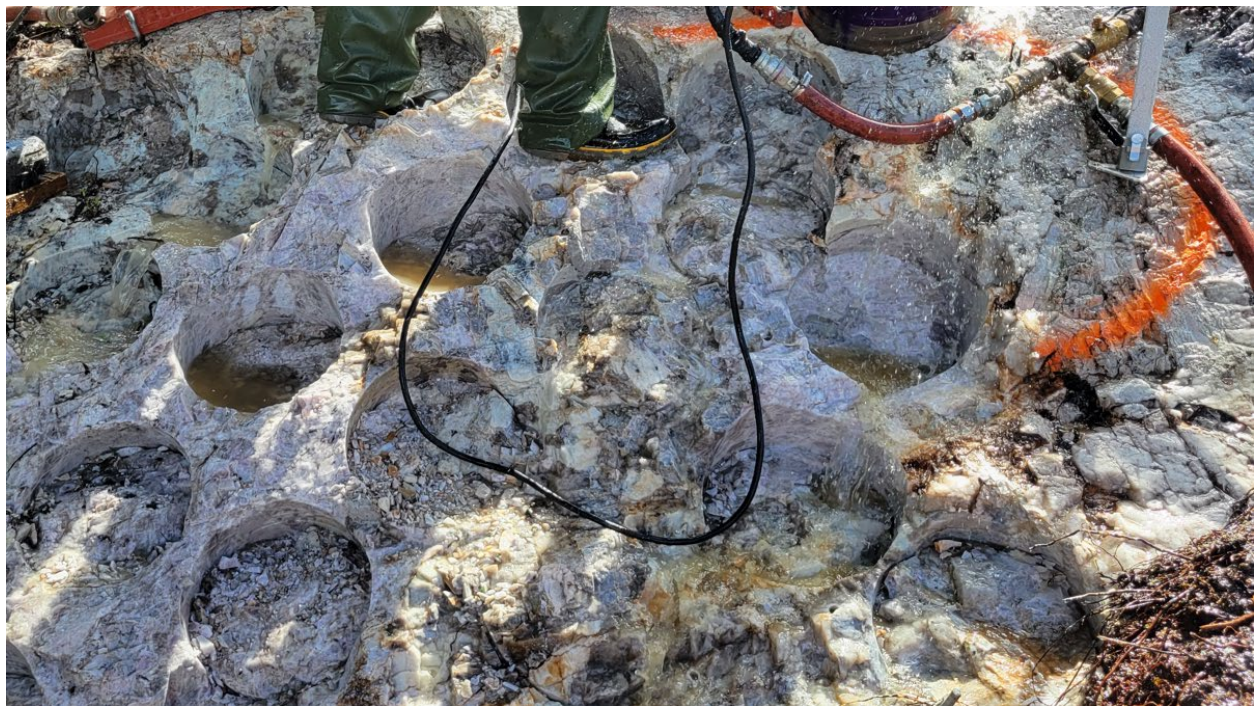
Figure 2: (TOP) Cored drill hole (~30 cm diameter) in pollucite pegmatite outcrop; (BOTTOM) Grid of cored drill holes (~30 cm diameter) in pollucite pegmatite outcrop (see Table I). Segments between holes are jackhammered out and added to sample composite.
