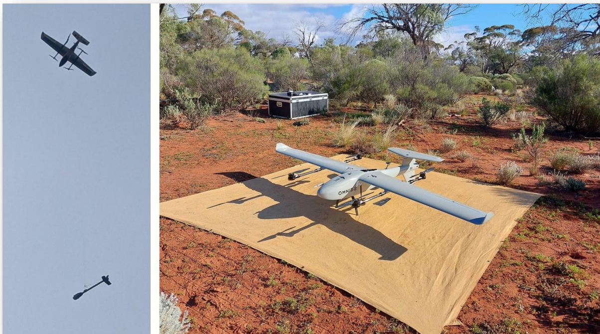
Figure 1: Drone magnetic survey at the Leonora Goldfields Project — the Shift Geophysics survey aircraft with towed-bird magnetometer in flight (left) and on the landing pad between flights (right).
