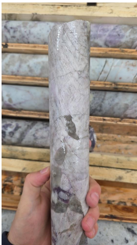
Figure 6: Geologist holding piece of core from spodumene pegmatite interval in hole BL26-030 at around 169 m. Pink mineral is single spodumene crystal. 2
