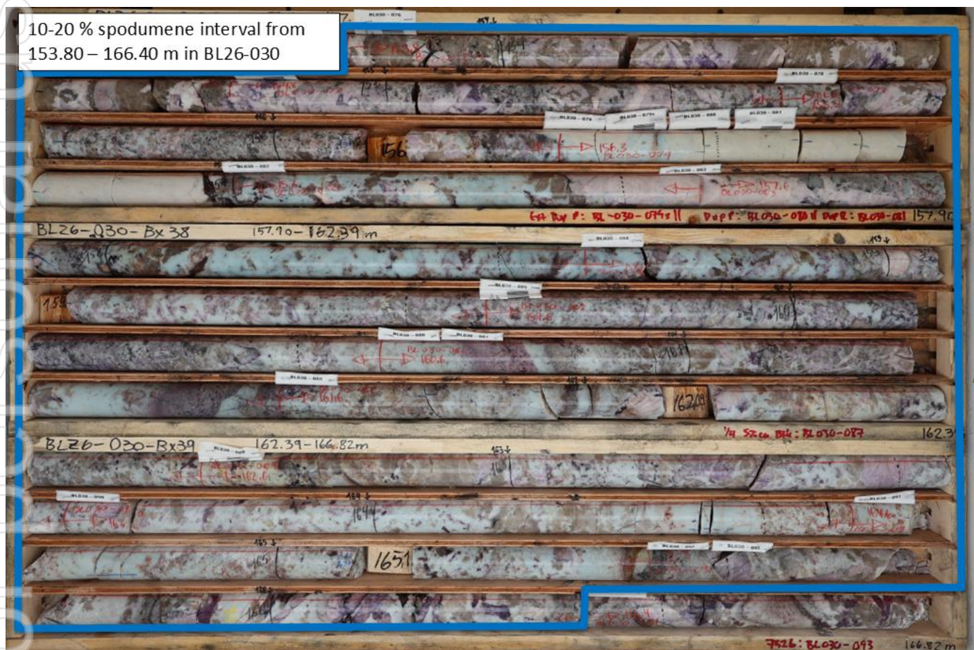
Figure 1: Spodumene pegmatite with visual estimates of 10-20 % spodumene from 153.80 – 166.40 m within larger interval in the first drill hole BL26-030 of 2026.
