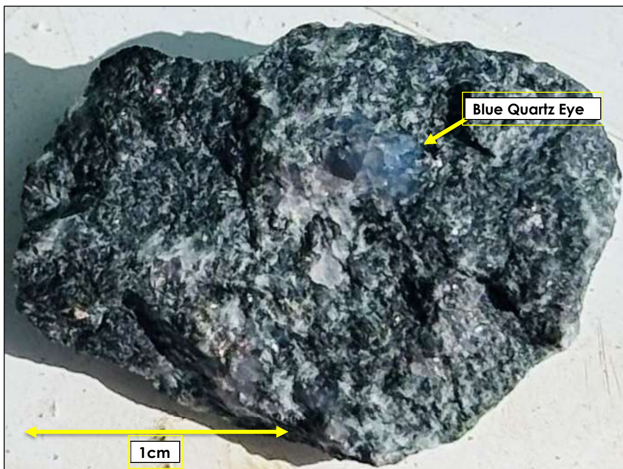
Figure 5: Selected example of a visually identified blue quartz eye within granophyric dolerite in 26MSRC005 at 99m, Mt Sandy.
