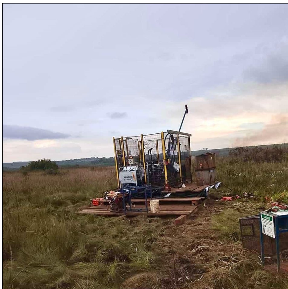
Photo 1: Diamond drill rig setup on first collar position targeting high-grade REE in the priority central corridor of the Serra Negra Carbonatite Complex.
